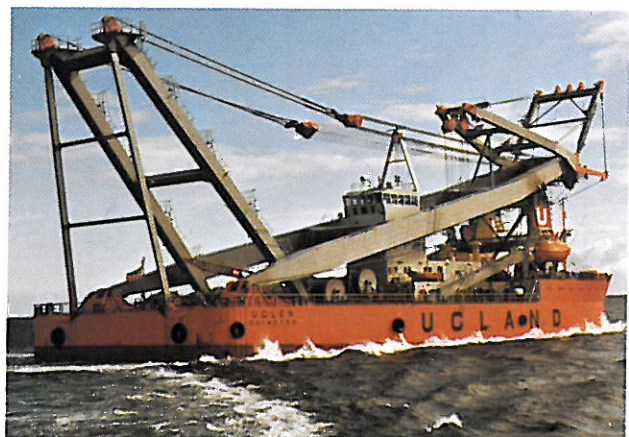
«UGLEN» with rig in transit position. At normal draft highest point will be 33 m above sea level with jib mounted and 28 m with jib dismantled.
