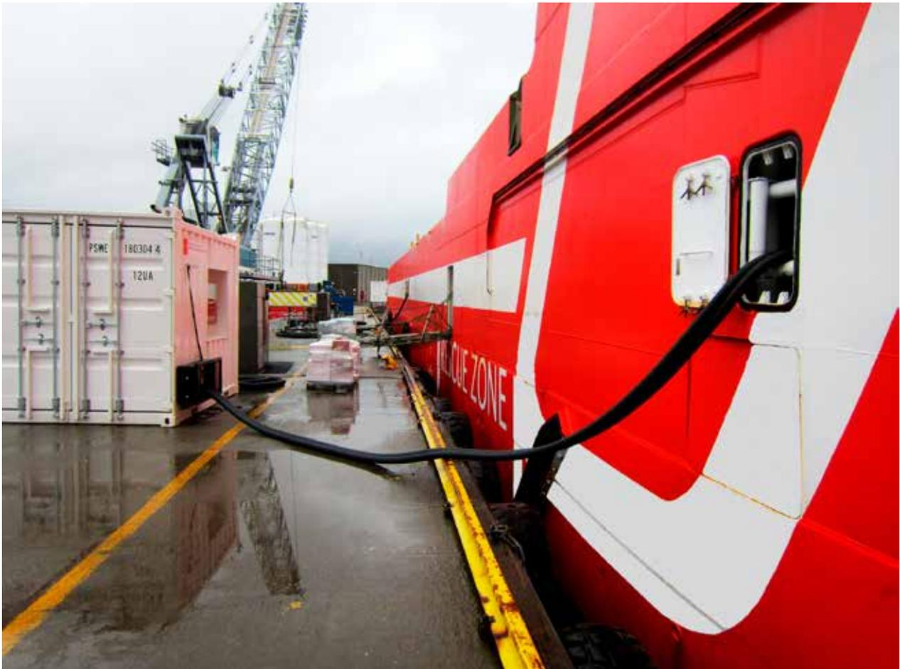
Shore connection cables connected at Mongstad base, supplying electric power to the ship while moored at quay
