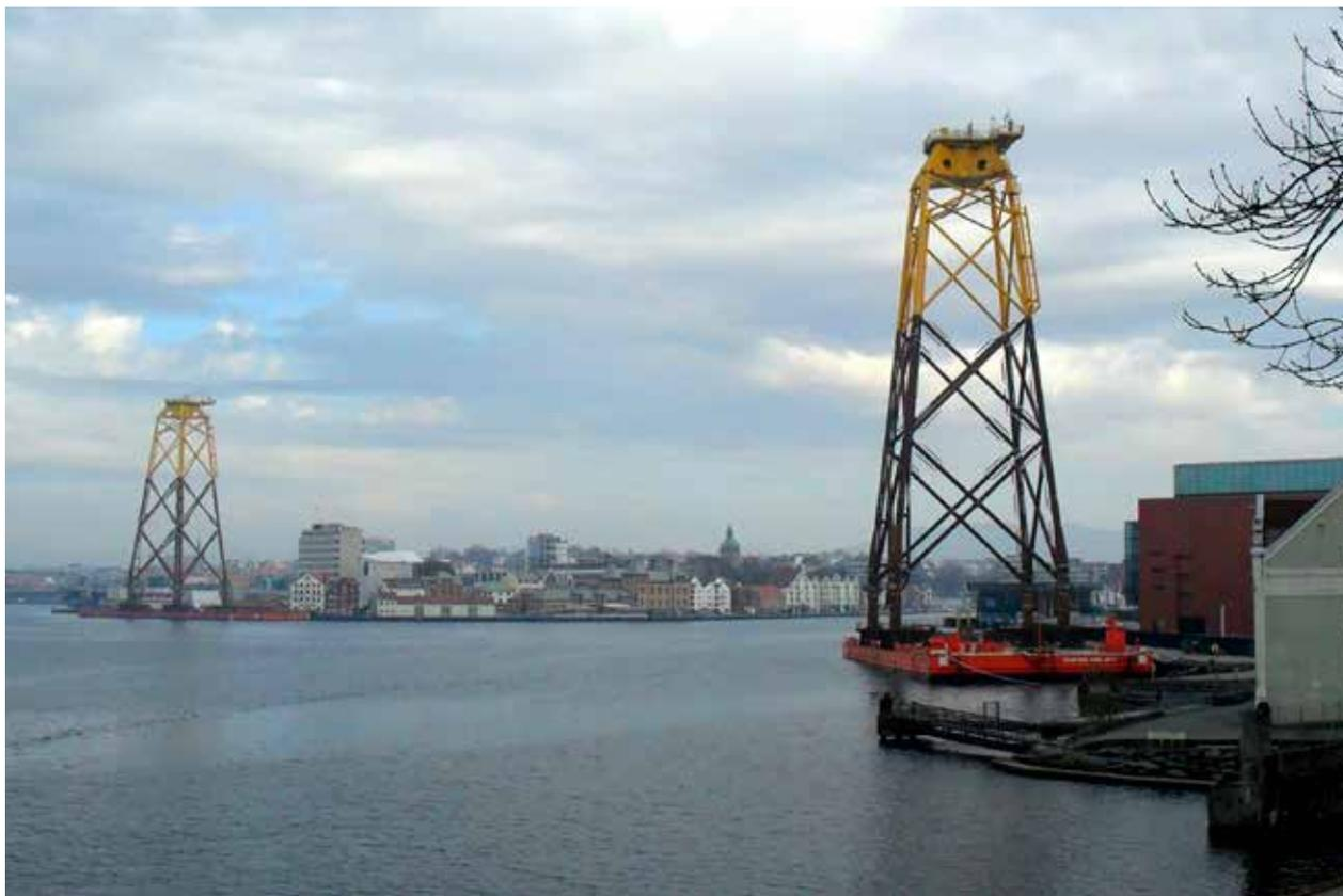
Transport of jackets for windmills; barge UR 99 to the left and barge UR 901 to the right
