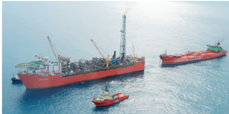
In this 2010 photo, the Mattea (right) offloads crude from the Terra Nova FPSO.
